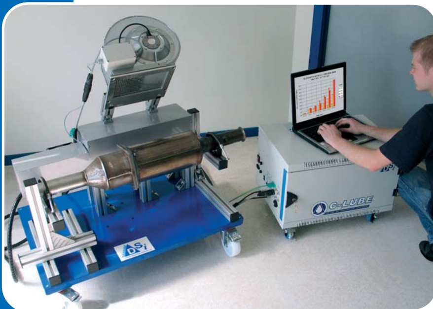
C-Lube, real-time oil consumption measurement on combustion engines
