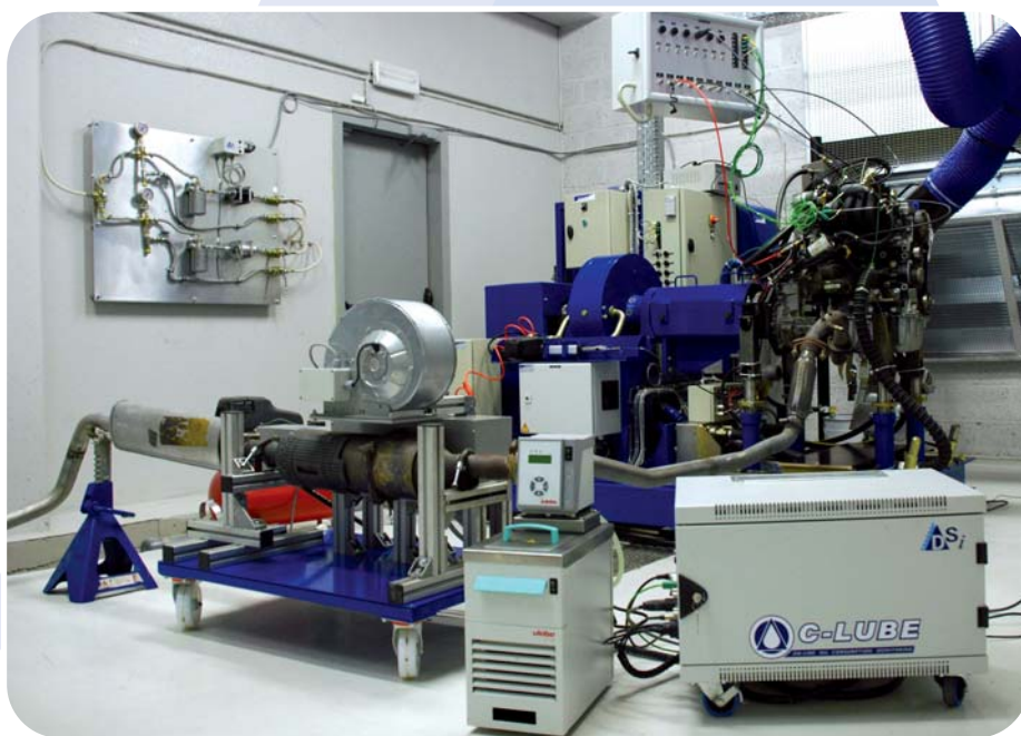
C-lube equipment installed in a test cell
