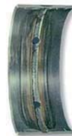
Bearing wear caused by a dilution problem
