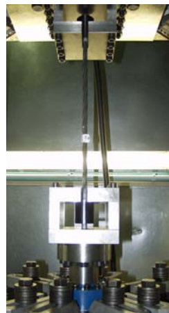
Reinforcing Steel Specimen
